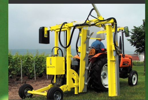
REAR MACHINES ON P.T.O. 2 complete rows – 2 half rows or 1 complete row.
