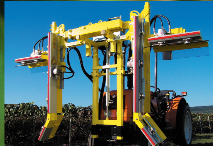
P2200 2 half rows at the front. 3 cylinders: 1 UP/DOWN – 2 IN/OUT. Exists with independent height adjustment.
