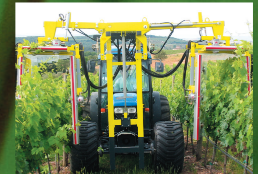
P3200 1 2 complete rows front mounted with up to 7 cylinders.
