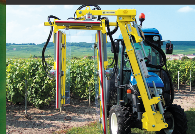
P3000 LZP Standard equipped with an oscillating frame with hydraulic parallelogram.
