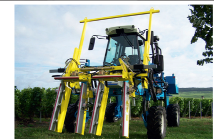
Vine trimmer on straddle tractors.
