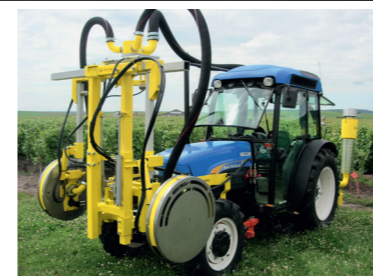
Leaf remover on inter-row tractors.
