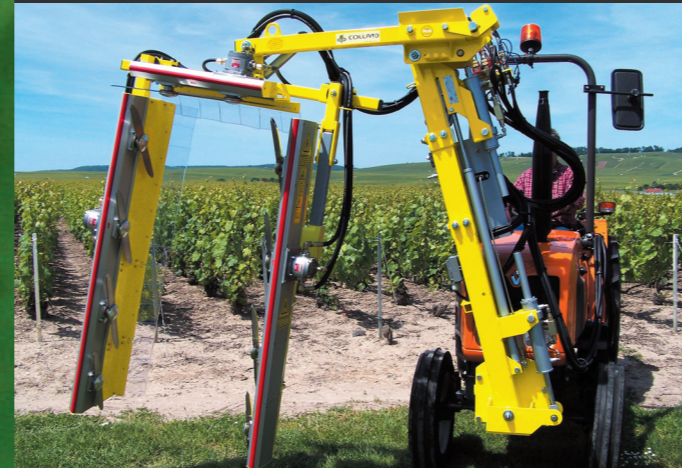
P3000 LZP Multi purpose Reinforced frame, 1 SE + 5 DE. Equipped with a fast fixing. This frame allows the fitting of the leaf remover.
