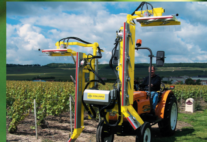
P2200 U 2 half rows at the front. 6 cylinders. Independent height adjustment & Exceptional forward visibility.
